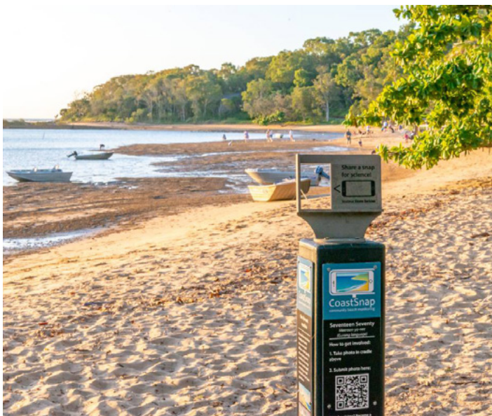
Beach monitoring. This is a “CoastSnap” station on the coast of Queensland, Australia, used to monitor beach levels (photo by Gladstone Regional Council).
