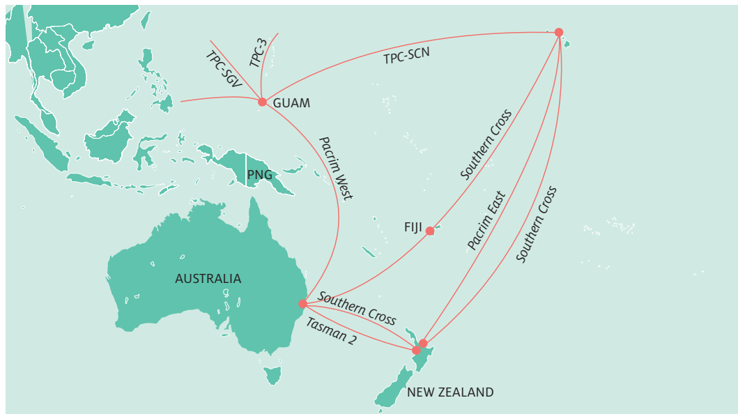
Figure 5. Fibre-Optic Cables Serving the South Pacific Region
